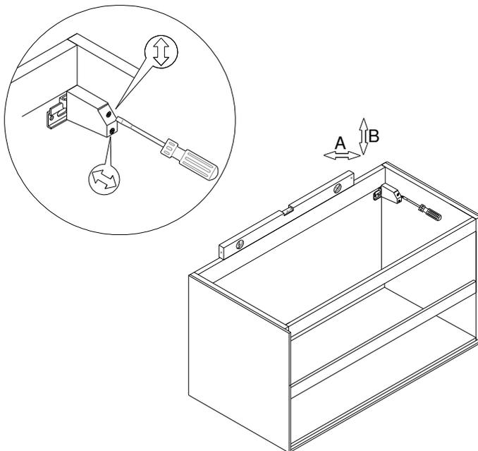
5) Adjust the height of the Vanity unit, turning the screw (B) of both supports till furniture is at right horizontal level. Hang the furniture, hooking the brackets onto wall-mounting plates and turn the screws (A) belonging to the furniture brackets.
