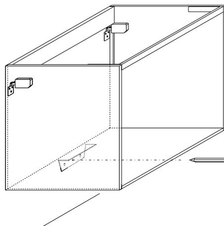
6) At the wall, please mark the points, where you will drill the holes, in order to fix the supporting "L" bar, holding the furniture.
