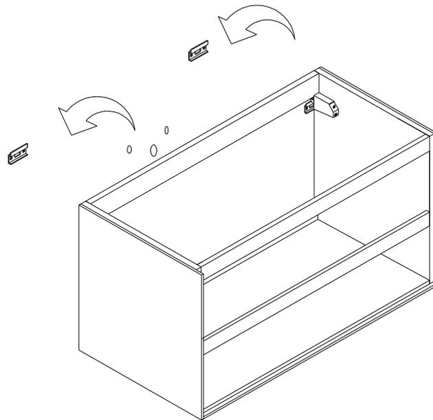
4) Hang the Vanity unit to the wall, by means of suitable wall brackets, which are already fixed at each side of the unit.
