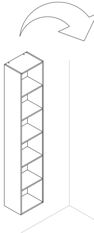
For your convenience it is recommended to unhook the cabinet from the wall, after marking the position of the holes.
