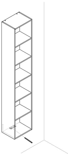
Draw at the wall the points, where you will drill the holes for the supporting bracket.
