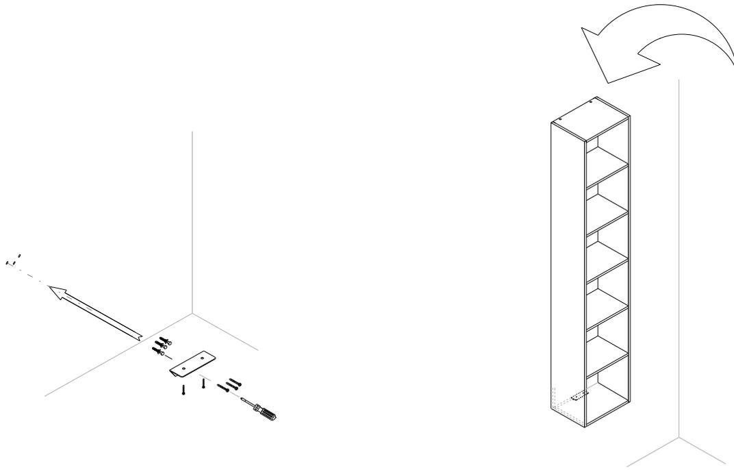
**Drill the holes with a drilling machine, where you marked the points. Insert the equipped dowels and fix the supporting bracket, screwing the equipped screws.**
