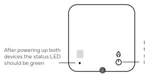
Press the manual override to check if the boiler switches on. Button LED lights green
